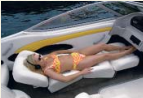
Adjustable Lounge Seats with Injection Molded Polypropylene Cores
