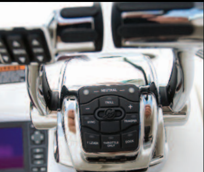
Digital Throttle and Shift (DTS) Provides effortless shifting and docking assistance.
