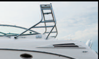
Radar/sport arch Convenient for mounting navigation equipment and electronics or for attaching a towrope.
