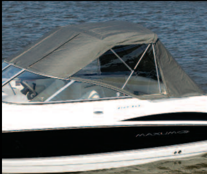
*Convertible top with side and aft canvas with enclosures Versatile and durable, this canvas option can simply cover or enclose the entire cockpit.
